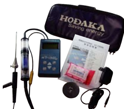
HT-1300N Standard set • Main unit • Sampling probe HT-1006 • Battery charger • Carrying case • Soft case • Reflection plate • Filter set • User manual Price 198,000yen (tax exclude)
